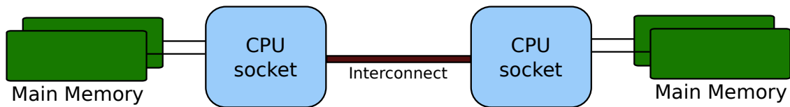
Fig. 4.2: Schematic of a two-socket NUMA system. Processes should be spread across both CPUs to obtain full bandwidth.
